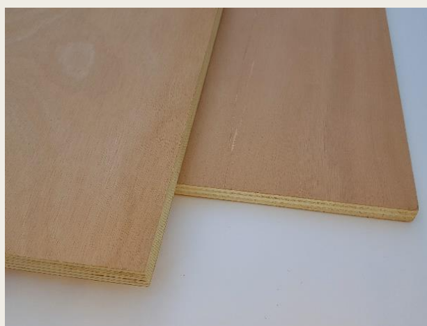
Photo: Inside and outside faces of plywood© M. Vernay
